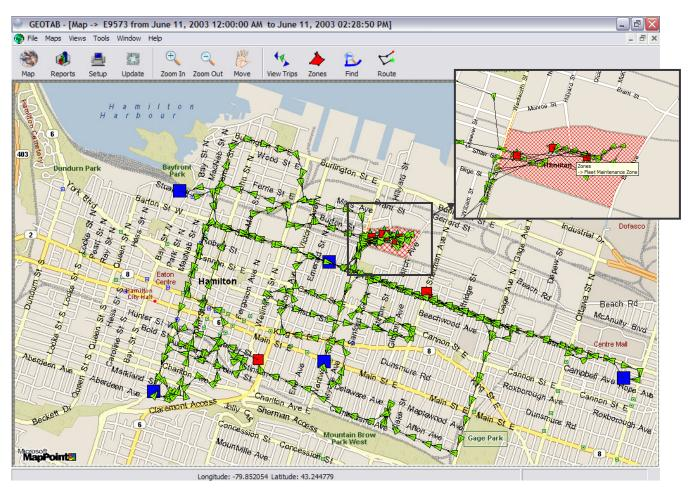
In this example, a street sweeper's trip for 1 day is shown on the map. GEOTAB uses a zone creation function to easily draw an area around the fleet facility for the city. Street sweepers regularly return to the facility throughout the day to empty the collected road debris. These return trips and time spent in the yard per trip can be viewed for over-idling.
